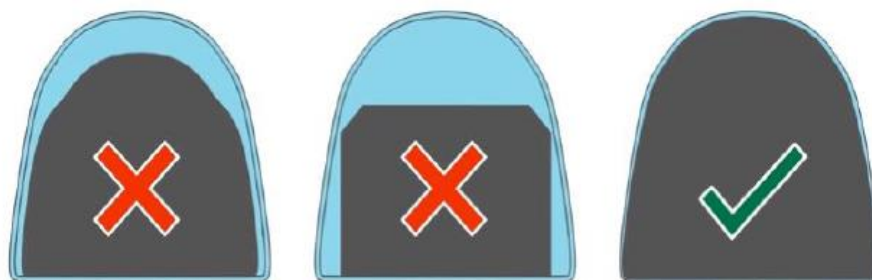
Figura 1.7 Cobertura ideal panel contra fuego Fuente: Shell Eco-marathon Tech Tips Vehicle Design [23].
