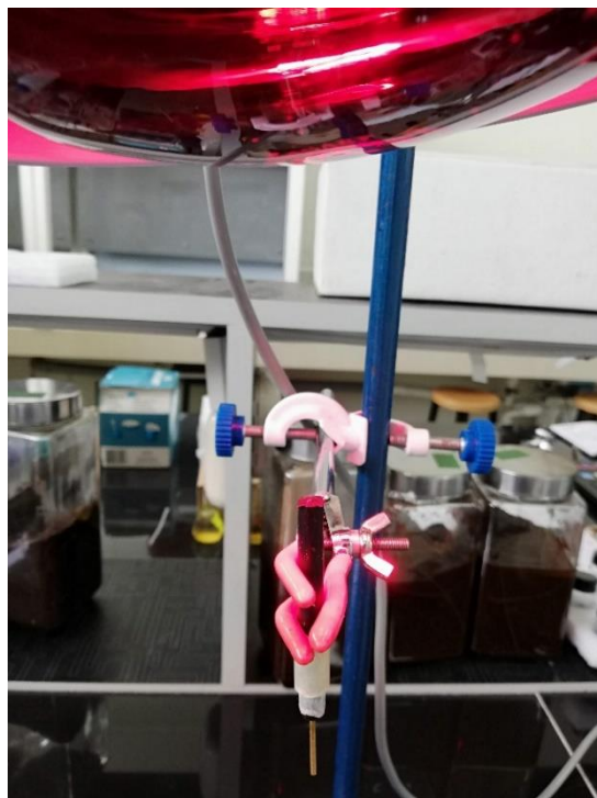
Figure 2.5. Silver nanoparticles ink drying by IR light over buckypaper pasted over glassy carbon work electrode
