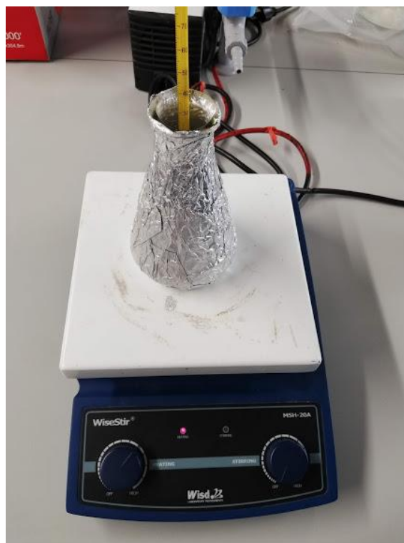
Figure 2.3. Erlenmeyer flask with a magnetic pill totally covered with aluminum foil being heated for the Frens method synthesis of silver nanoparticles. Source: Own elaboration.
