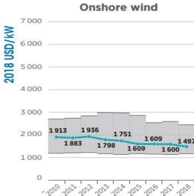
Figura 2.4 Global weighted average total installed costs for Onshore Wind 2010-2018 Fuente: IRENA. Renewable Power Generation Costs in 2018 [60]
