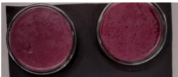
Figure 7.10. Left: pre-treatment control, right: electroporated sample after treatment.
